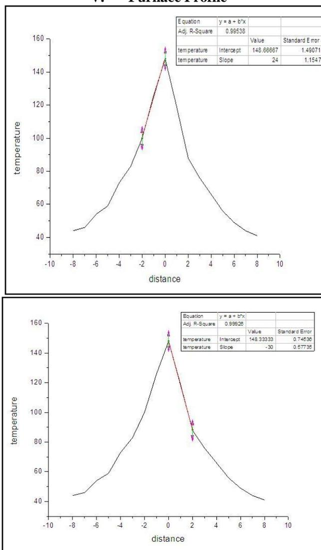
Temperature gradient is  $24^{\circ}\text{C}/\text{cm}$  on one solid-liquid interface and  $30^{\circ}\text{C}/\text{cm}$  at the other interface. Molten-Zone length was 4-5 mm.
