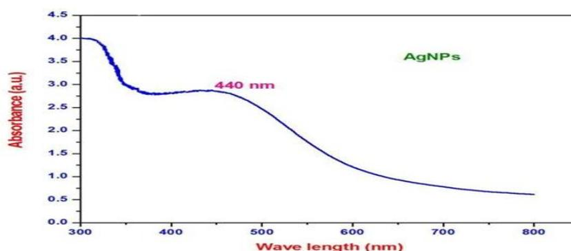
Figure.1 UV-Visible spectrum of biosynthesized AgNPs using *Dodonaea viscosa* leaf extract.
