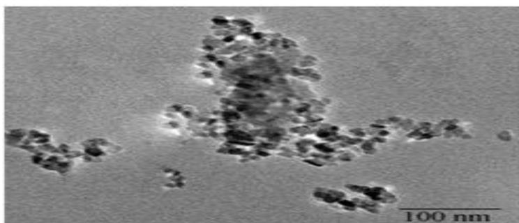
Figure.4 TEM image of biosynthesized AgNPs using *Dodonaea viscosa* leaf extract.
