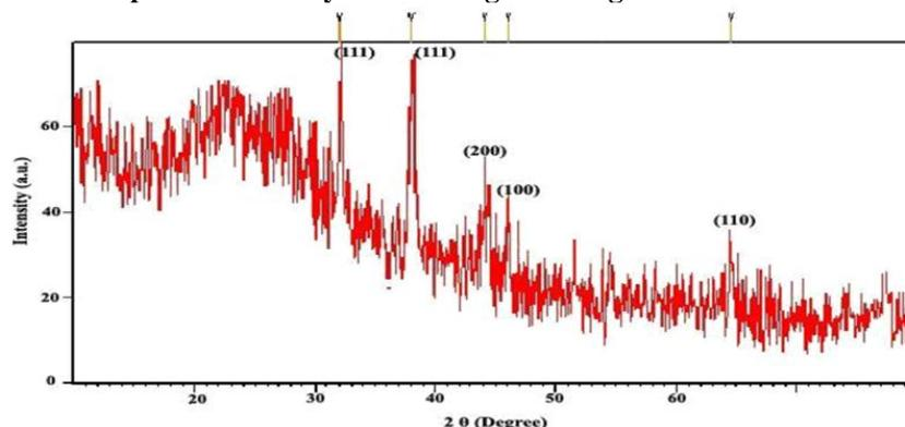
Figure.3 XRD pattern of biosynthesized AgNPs using *Dodonaea viscosa* leaf extract.
