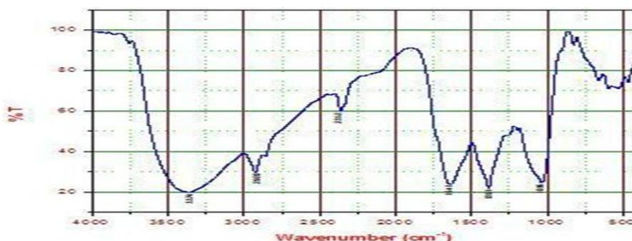
Figure.2 FTIR spectrum of biosynthesized AgNPs using *Dodonaea viscosa* leaf extract.
