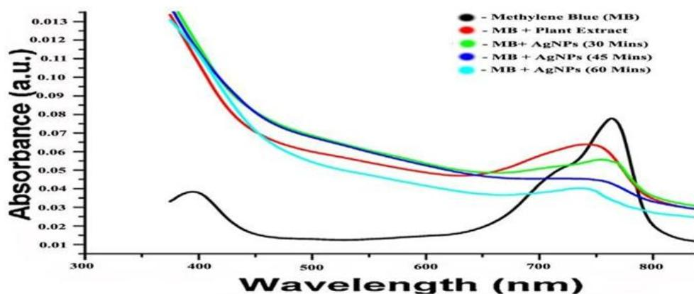
Fig. 6 UV-Vis spectra of methylene blue degradation test for catalytic assay
