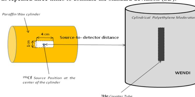
**Figure 2:** Experimental setup arrangement to measure the dose rate by Wide Energy Neutron Detector Instrument (WENDI).
