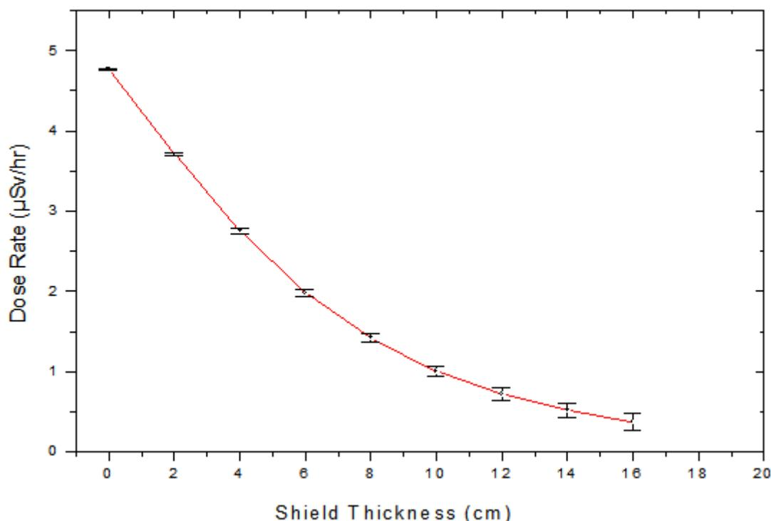
Figure 3: Neutron dose rate calculated by MCNP5 model.
