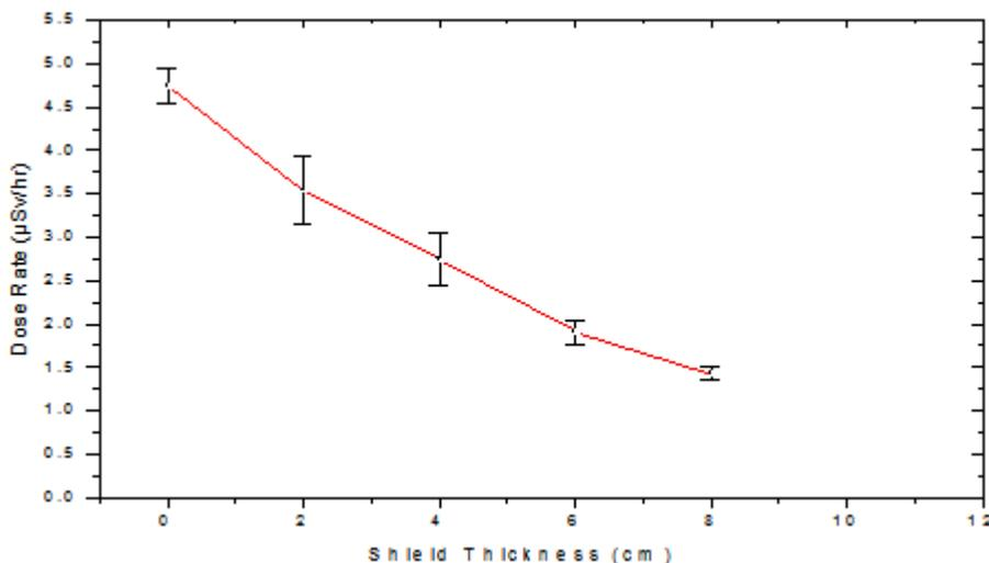
**Figure 4:** Neutron dose rate measured by Wide Energy Neutron Detector Instrument (WENDI).
