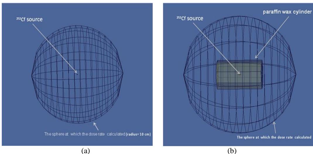
**Figure 1:** Neutron source and cylinder Containing  $^{252}\text{Cf}$  source Generated by MCNP Visual Editor. (a) Neutron source in air (without shield) (b) Paraffin wax cylinder containing  $^{252}\text{Cf}$  source.
