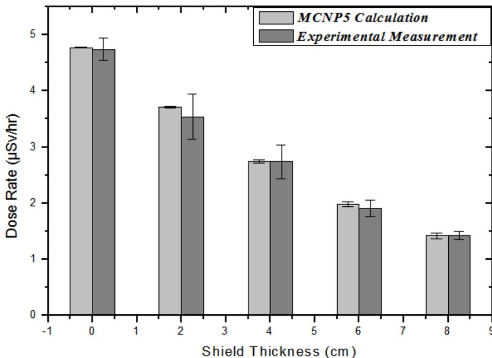
**Figure 5:** Neutron dose rate calculated by MCNP5 model in comparison with that measured by Wide Energy Neutron Detector Instrument (WENDI).
