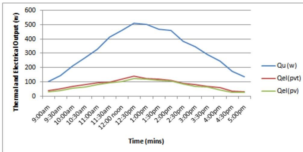
**Figure 5:** Variation of  $Q_u$ ,  $Q_{el}$  (pvt) and  $Q_{el}$  (pv) vs. time for a sunny day (12<sup>th</sup>, May 2014)
