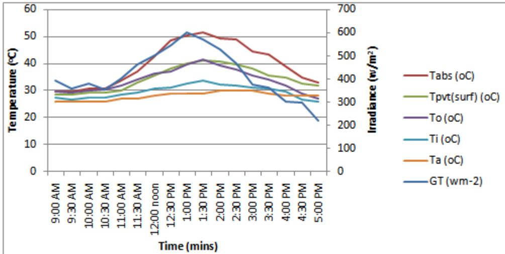
**Figure 4:** Time series of the monitored parameters on a cloudy day (19<sup>th</sup>, May 2014).
