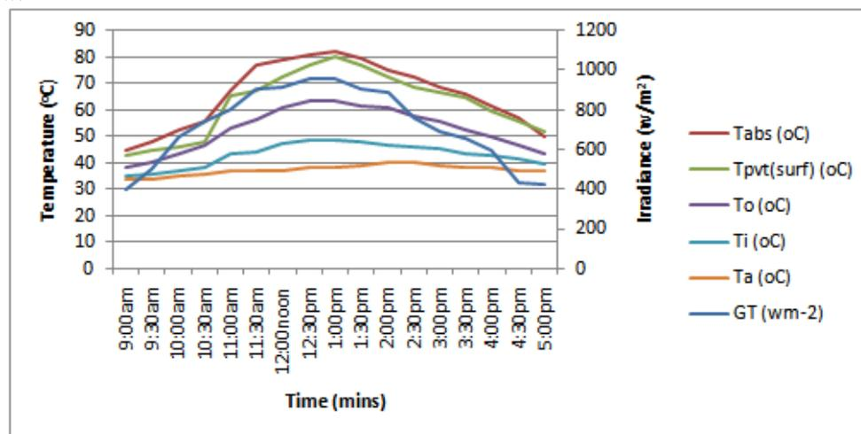
Figure 3: Time series of the monitored parameters on a sunny day (12<sup>th</sup>, May 2014)
