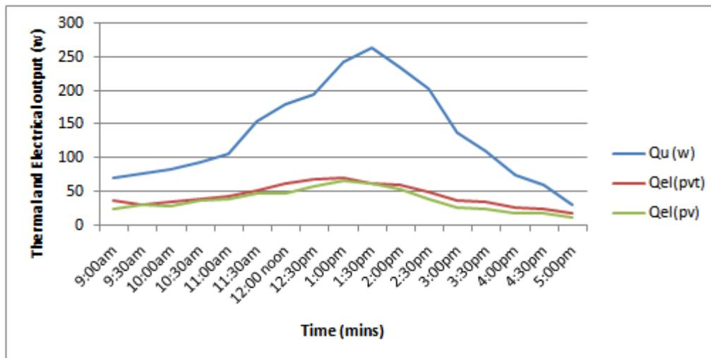
**Figure 6:** Variation of  $Q_u$ ,  $Q_E$  (pvt) and  $Q_E$  (pv) vs. time for a cloudy day (19<sup>th</sup>, May 2014)
