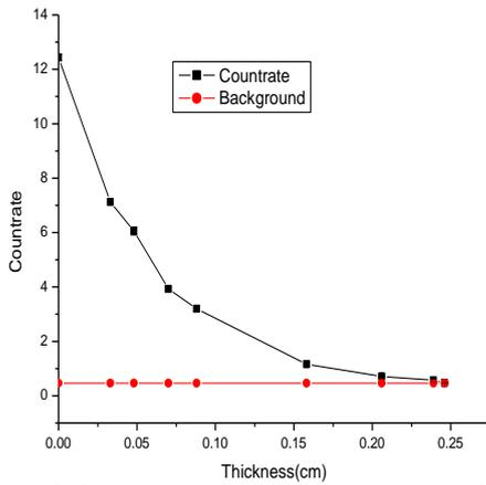
Fig.(2): Plot of count rate v/s Thickness for paraffin wax with Tl- 204 source.
