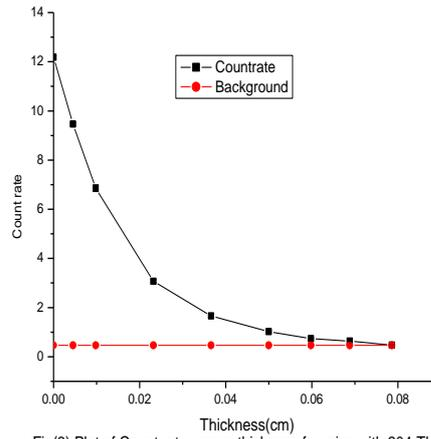
Fig(3):Plot of Count rate versus thickness for mica with 204-Tl beta source
