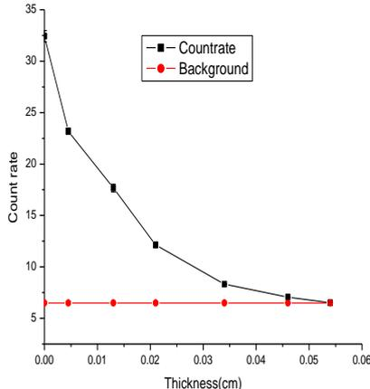
Fig.(5) Plot of count rate versus thickness for mica with Cs-137 beta source.
