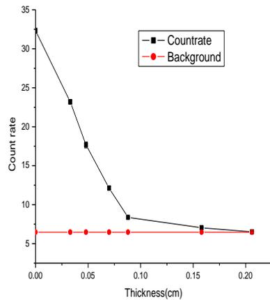
Fig.(4) Plot of count rate versus thickness for paraffin wax with 137Cs beta source.
