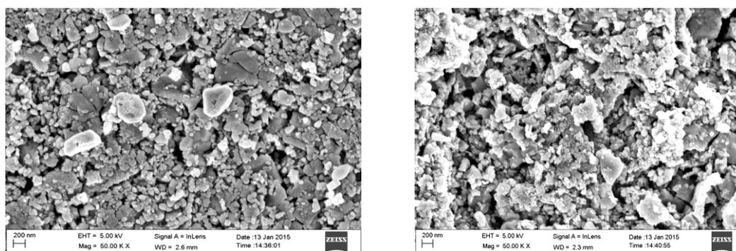
Fig (3) FESEM micrographs of Cu Substituted Mg-Zn ferrites
