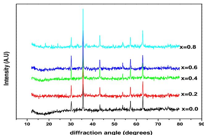
Fig(1). XRD pattern of Cu Substituted Mg-Zn ferrites
