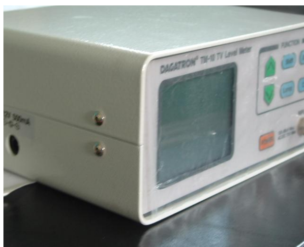
Fig 3a: The Dagatron T M10 Field Strength Meter. Fig. 3b: Global Positioning System (GPS) Receiver GARMIN MAP 76 personal navigator
