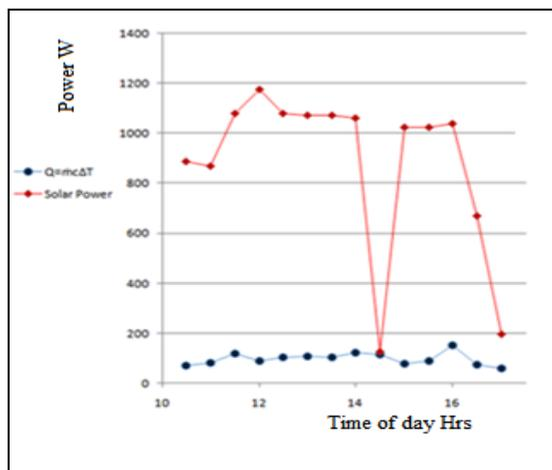
**Figure 9:** Performance of Non-Compensated Absorber
