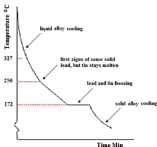
**Figure 2:** Cooling curve of 60Sn40Pb alloy [Source -www.chemguide.co.uk]
