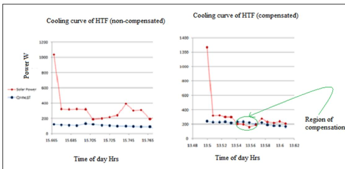
Figure 10: Comparing cooling curves of compensated and non-compensated absorbers
