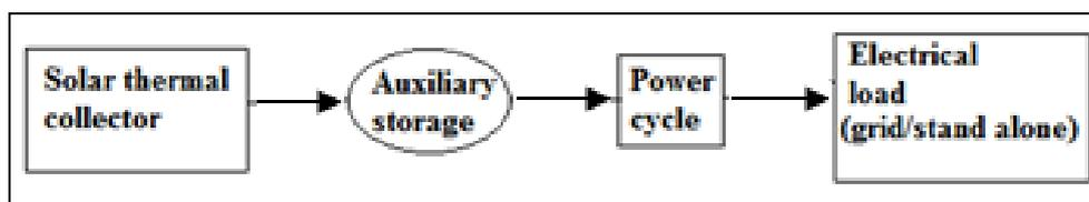
**Figure 3:** Schematic diagram representing solar energy transformation
