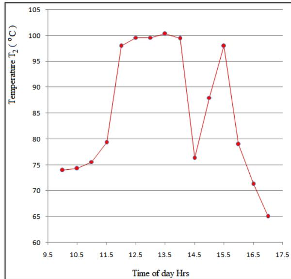
Figure 7: Output temperature variation of HTF
