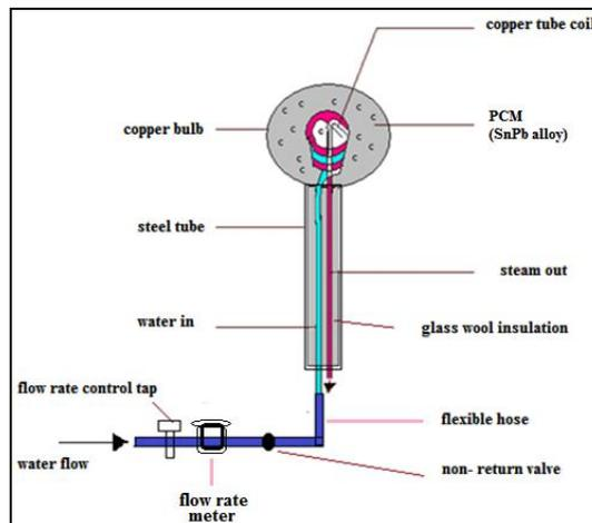
Figure 4: Components of the compensating absorber
