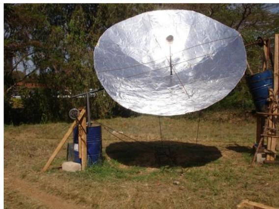
Figure 6: The complete PDSC assembly
