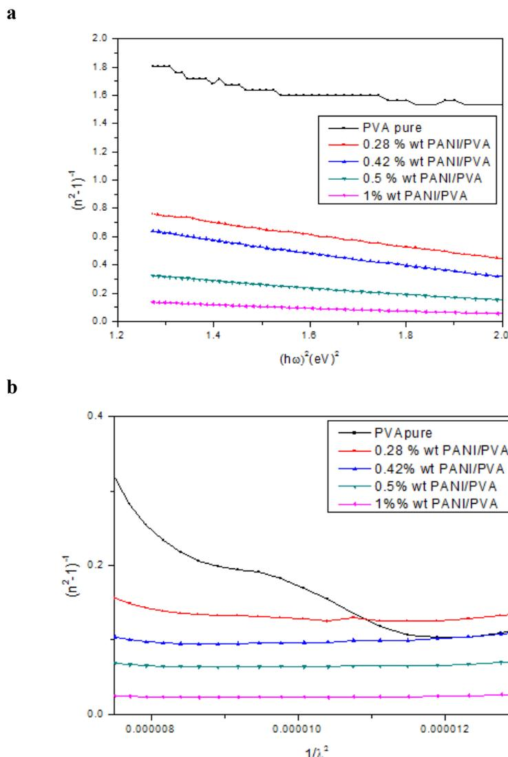
Fig (7) Plots of (a)  $(n^2-1)^{-1}$  vs.  $(h\omega)^2$  (b)  $(n^2-1)^{-1}$  vs.  $(1/\lambda^2)$  for pure PVA and PANI/PVA blends.
