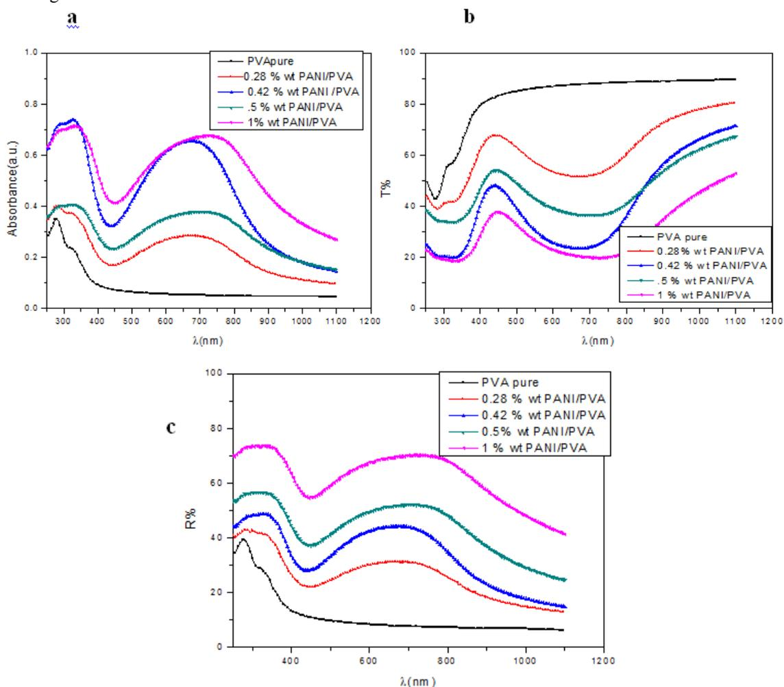
Fig (3) (a) Absorption, (b) transmission and (c) reflectance spectra as a function of wave length for PANI /PVA blend films.
