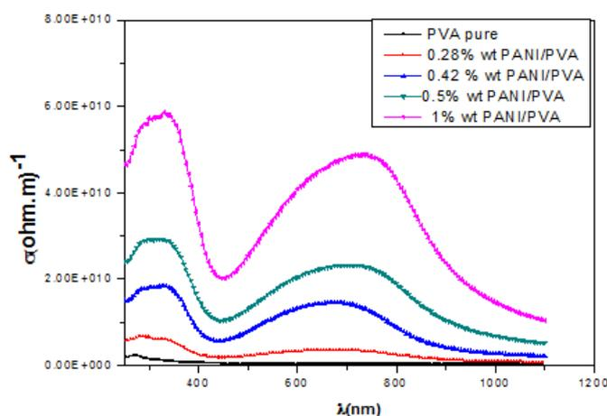
Fig (9) shows the variation of optical conductivity with wavelength for PVA pure and PANI/PVA blend.
