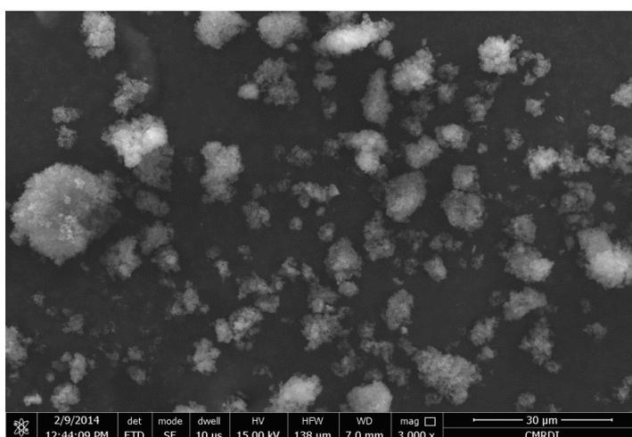
Figure 2: SEM micrograph of polyaniline (EB) powder.
