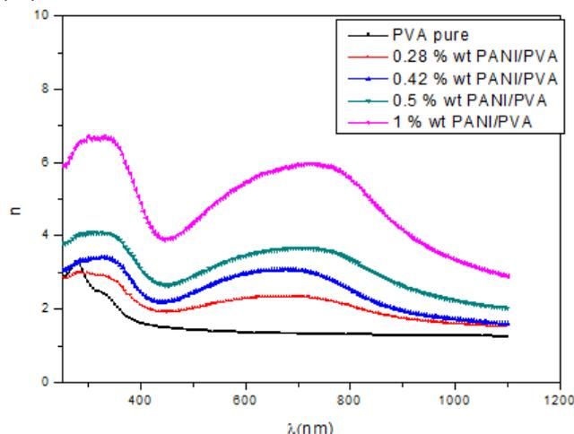
**Fig (5) The refractive index of PANI/PVA blend at different concentration of PANI.**
