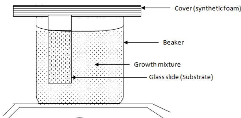
Fig. 1. Experimental set up.
