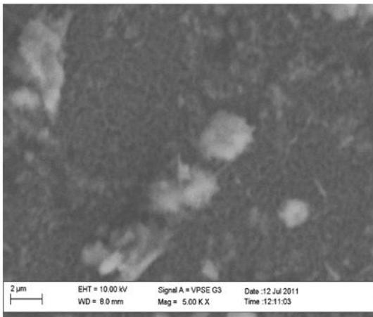
Fig.1a: SEM of as-deposited NiSe film
