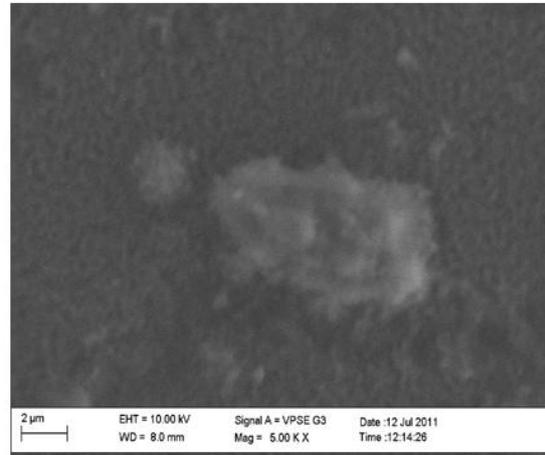
Fig.1b- SEM of NiSe film annealed at 100° C
