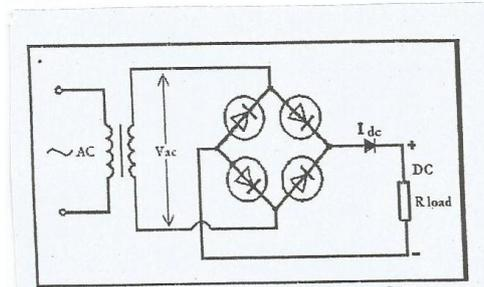
**Figure 2: The Bridge rectified circuit**
