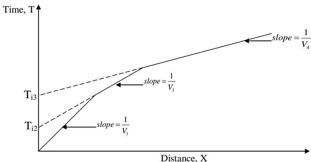
Fig. 2: Time distance graph of a four layer case seismic refraction survey, where the second layer with velocity  $v_2$  was undetected.
