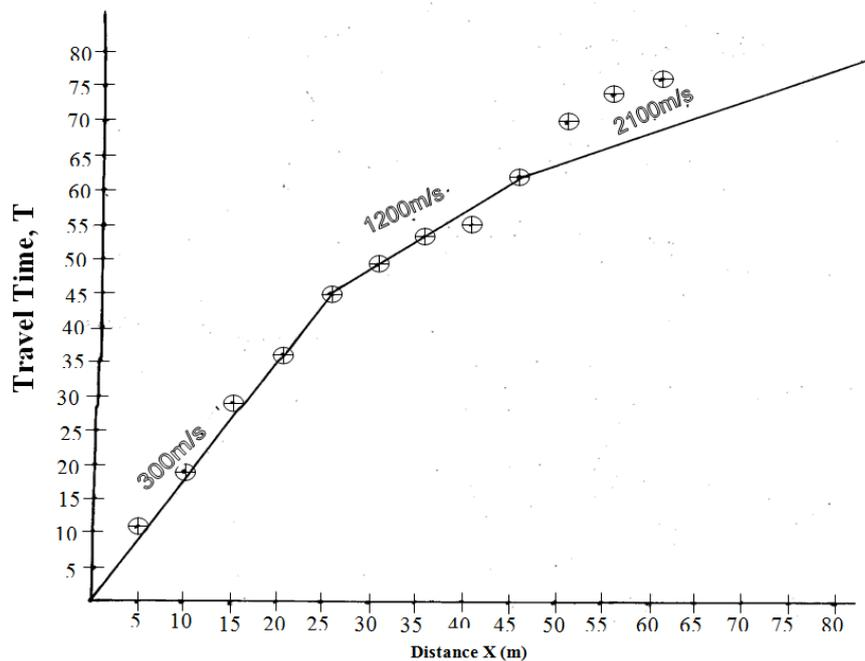
Fig. 3: T-X plot of Seismic refraction data obtained from the study area.
