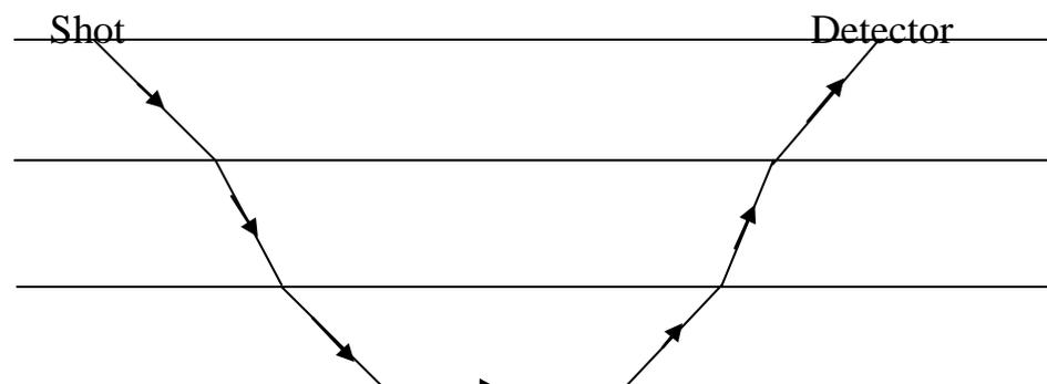
Fig. 1: Refraction paths of travel time-distance curves when a low-velocity layer  $V_1$  lies below a higher-speed layer,  $V_2 > V_3 > V_4$
