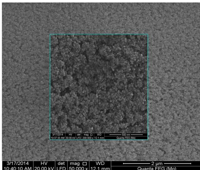
Figure 1. Top view FE-SEM images of the nanostructured CdS thin film deposited onto a glass substrate.
