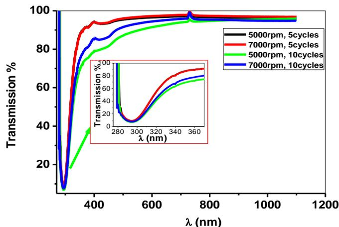
**Figure 3. Transmittance spectra of nanostructured CdS thin films with different thicknesses.**
