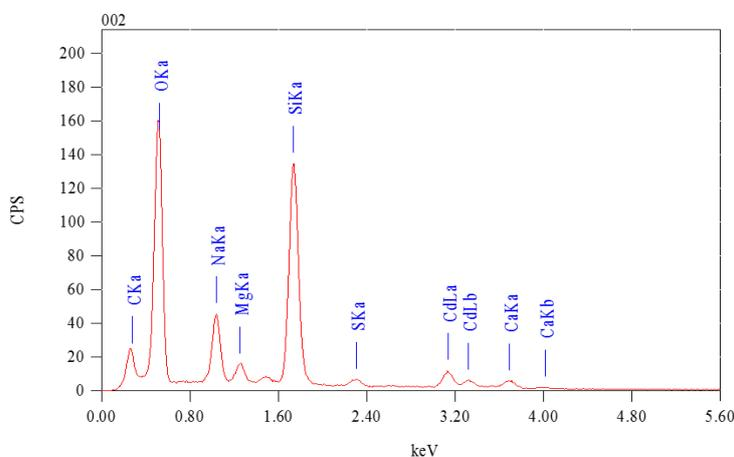
Figure 2. EDX spectra of spin coated nanostructured CdS thin film.
