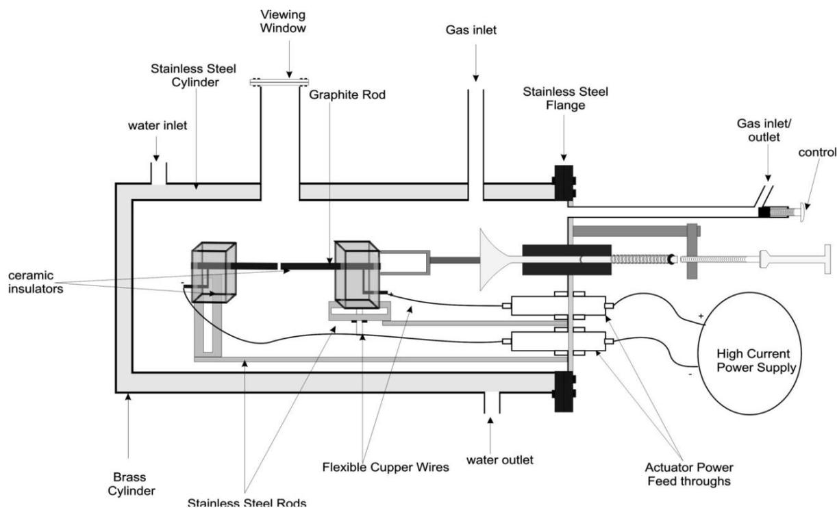
**Figure 3:** Arc discharge system for fullerenes synthesis
