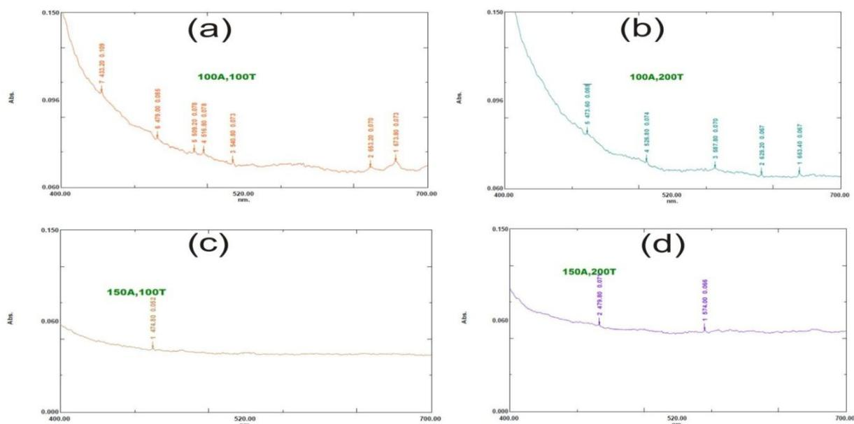
**Figure 5:** UV-Vis Spectra of fullerenes solid extracted from carbon soot collected at different arc discharge operating conditions of discharge current and chamber pressure of (a) 100 A and 200 Torr (b) 100 A and 200 Torr (c) 150 A and 100 Torr (d) 150 A and 200 Torr.
