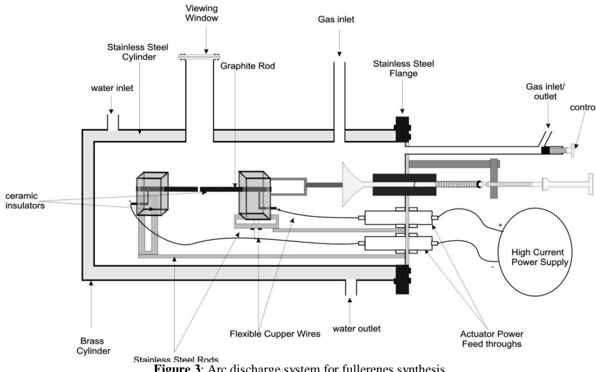
**Figure 3:** Arc discharge system for fullerenes synthesis
