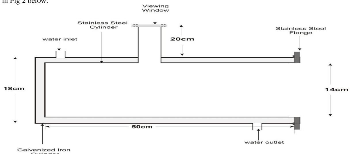
**Figure 2:** fabricated double walled cylinder with a viewing window
