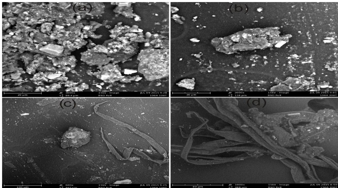
**Figure 4:** SEM Images of fullerenes solid extracted from carbon soot collected at different arc discharge operating conditions of discharge current and chamber pressure of (a) 100 A and 200 Torr (b) 100 A and 200 Torr (c) 150 A and 100 Torr (d) 150 A and 200 Torr.
