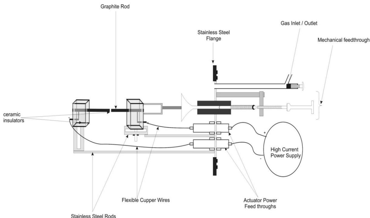
**Figure 1:** Flange carrying all components required inside the arc discharge chamber
