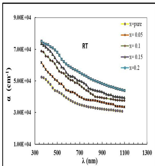
Figure(4) The variation of with absorption coefficient wavelength for TiO<sub>2</sub>:CuO thin films at RT with at different of CuO (0,5,10,15,20) % wt .
