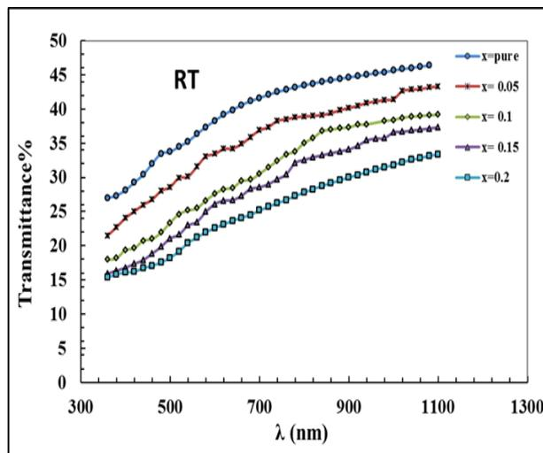
Figure(3) The variation of transmittance with wavelength for TiO<sub>2</sub>:CuO films at RT with different concentration of CuO ( 0, 5, 10, 15 and20) % wt.
