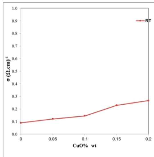
Fig(8) Variation of DC Conductivity at RT with CuO for TiO<sub>2</sub>:CuO thin films at RT with at different concentration of CuO (0,5,10,15,20) % wt .
