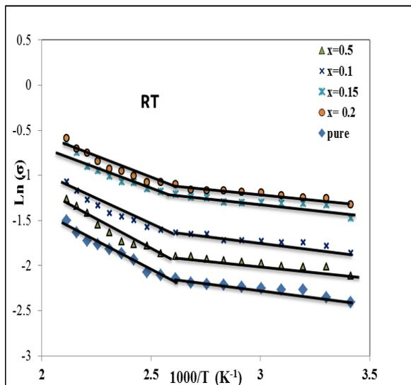
Fig (7) Variation of Ln(  $\sigma$  ) with reciprocal temperatures for TiO<sub>2</sub>:CuO thin films at RT with at different concentration of CuO (0,5,10,15,20) % wt .
