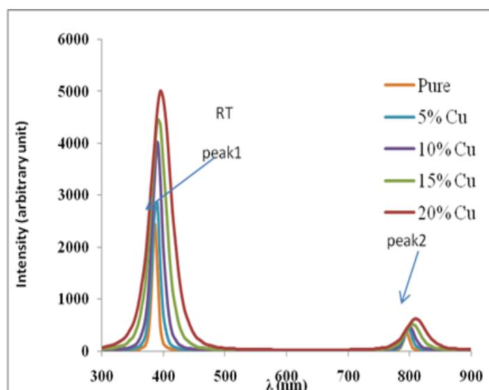
Fig (6): Room temperature photoluminescence spectra of the TiO<sub>2</sub>:CuO thin film at different concentration of CuO
