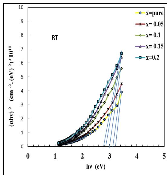
Figure(5) The variation of (αhv)<sup>2</sup> versus photon energy of (hv) for TiO<sub>2</sub>:CuO thin films at RT with at different of CuO (0,5,10,15,20) % wt .
