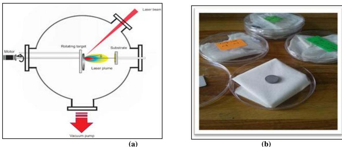
Fig (1) (a) Schematic of PLD [10],(b) palette of TiO<sub>2</sub>:CuO
