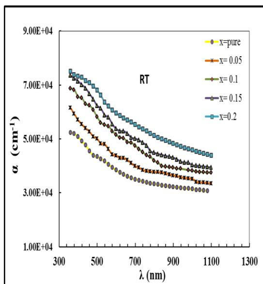
Figure(4) The variation of with absorption coefficient wavelength for TiO<sub>2</sub>:CuO thin films at RT with at different of CuO (0,5,10,15,20) % wt .
