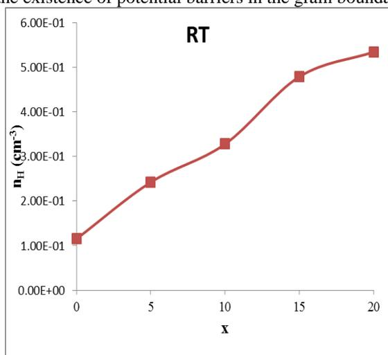
Figure(10)Variation of carrier concentration( $n_H$ ) with different concentration of CuO (0,5,10,15,20) % wt.
