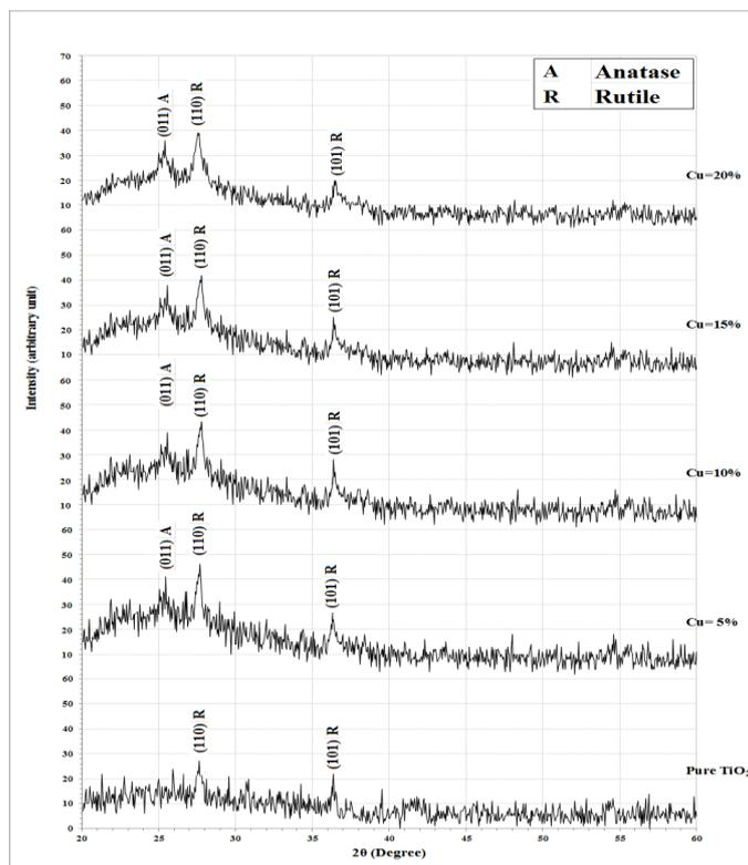
Fig. ( 2 ) X-ray diffraction patterns of as deposited TiO<sub>2</sub> films at 423K with different CuO doping ratio ( 0, 5, 10, 15 and 20) % wt
