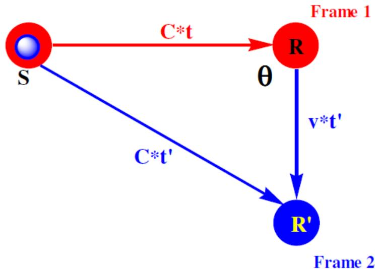
Figure 2. Receiver motion relative to the light path
