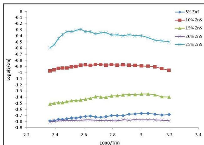
Fig.3. Electrical conductivity of PANI/ZnS Nanocomposite with different wt % of ZnS.
