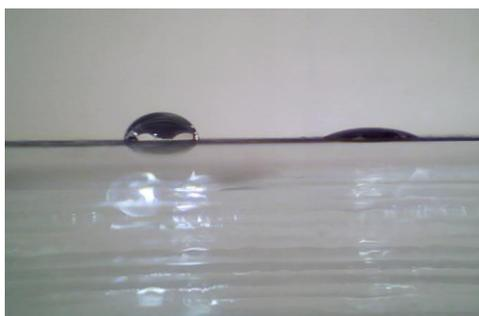
**Figure 2:** Photography of "A Droplet" of distilled water and ethylene glycol on the film of PANI-H<sub>2</sub>SO<sub>4</sub> which was formed from a solution synthesized at 20°C and at a speed of 6000 rpm
