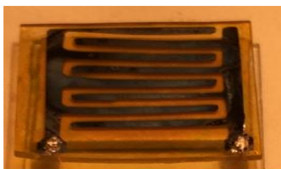
Fig. 1. PVD Electrodes on CdS thin film at 300c
