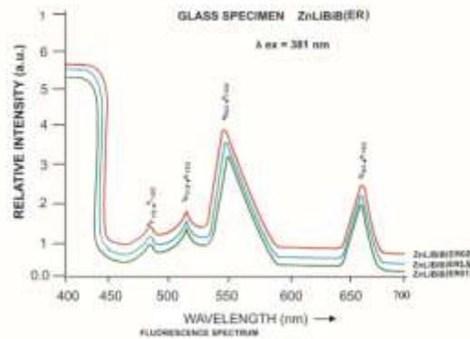
**Fig.3:** Fluorescence spectrum of ZnLiBiB glasses doped with Er<sup>3+</sup>.
