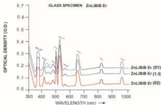
**Fig.2:** Vis-NIR absorption spectra of ZnLiBiB (ER) glasses.
