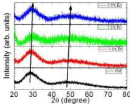
**Fig.1:** X-ray diffraction pattern of ZnLiBiB (ER) glasses.
