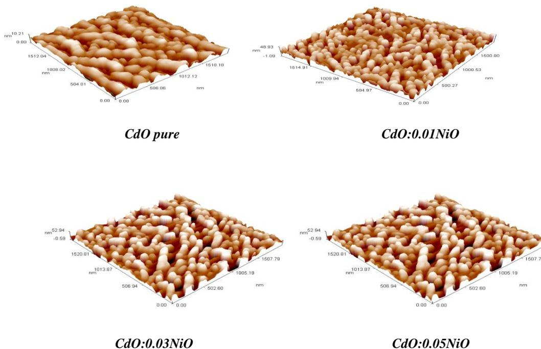
**Fig2:** Atomic force microscopy for CdO pure and CdO:NiO with different concentration at 723K
