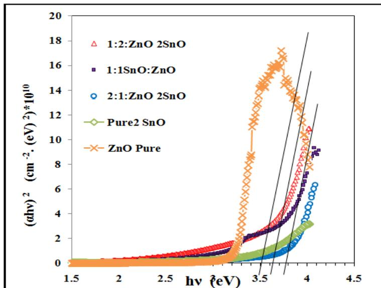
Fig.10: Optical band gap for ZnO/SnO<sub>2</sub> pure and their composition thin films deposited with different percentage.
