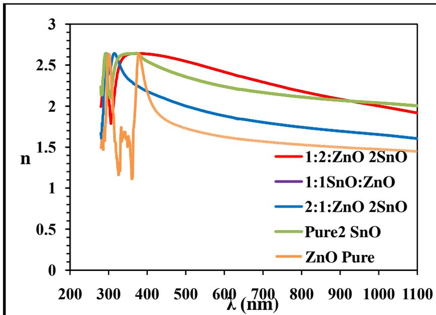
Fig.8. Reflective index spectra of ZnO/SnO<sub>2</sub> pure and their composition thin films deposited with different percentage.
