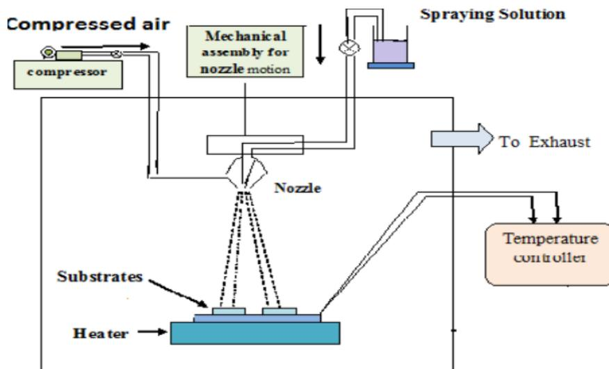
Figure (1) Schematic set-up for spray pyrolysis technique.
