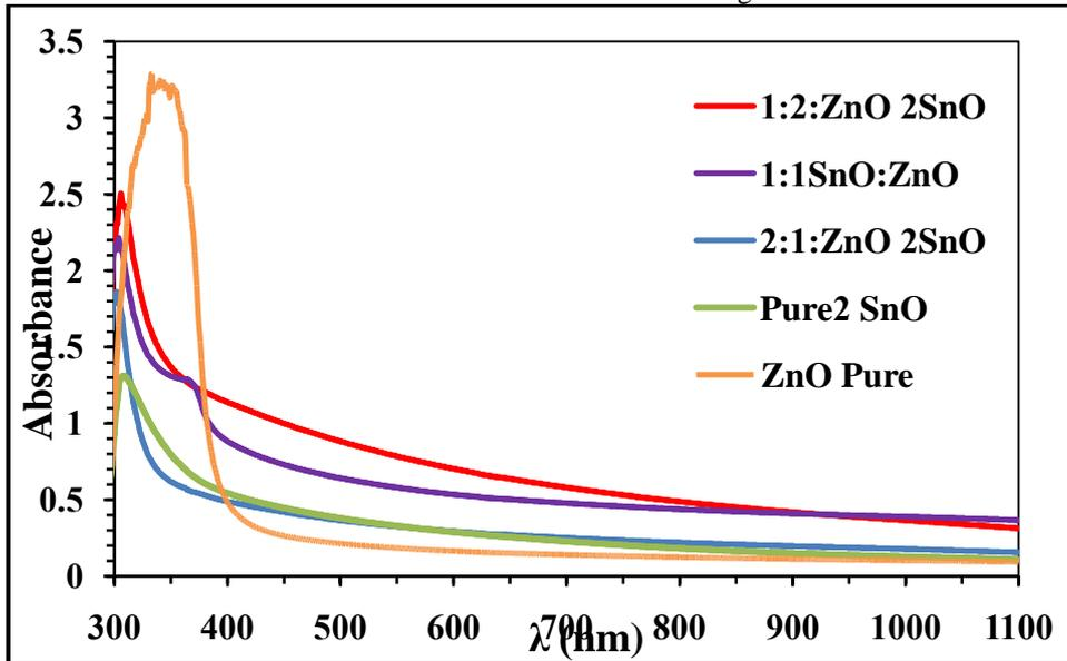
Fig.7: Absorption spectra for ZnO/SnO<sub>2</sub> pure and their composition thin films deposited with different percentage.
