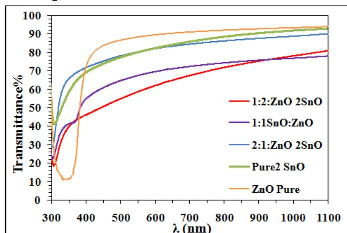
Fig.6. Optical transmission spectra of ZnO/SnO<sub>2</sub> pure and their composition thin films deposited with different percentage.
