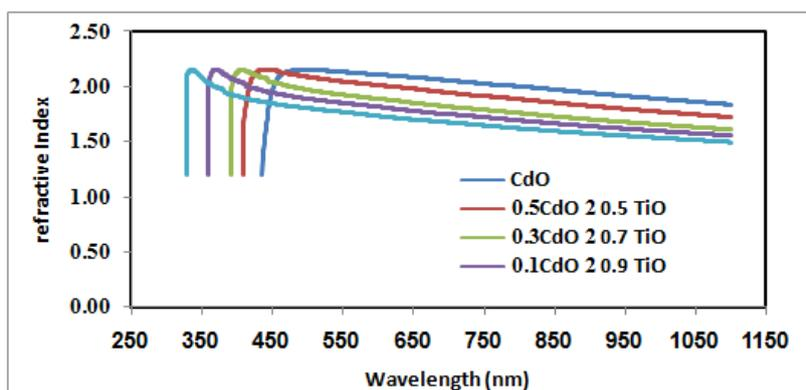
Fig.(6) :Variation of Refractive Index as a function of wavelength for  $(TiO_2)_{1-x}(CdO)_x$  films at  $T_a = 500 k$
