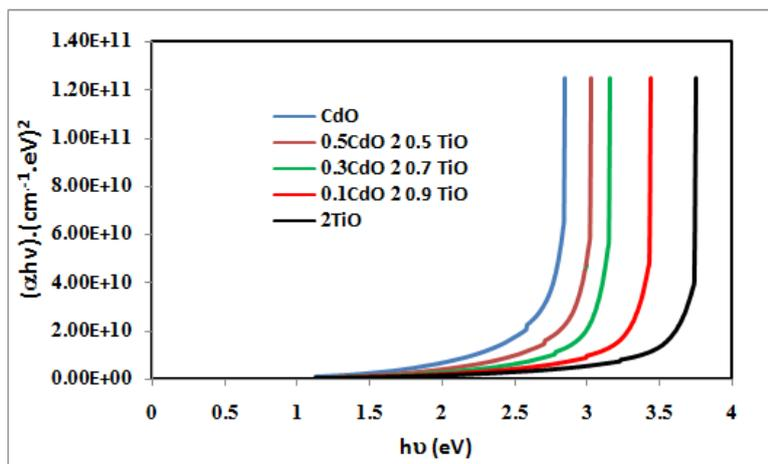
Fig.(5) : $(\alpha hv)^2$  as a function of  $h\nu$  for  $(TiO_2)_{1-x}(CdO)_x$  films at  $T_a = 500k$
