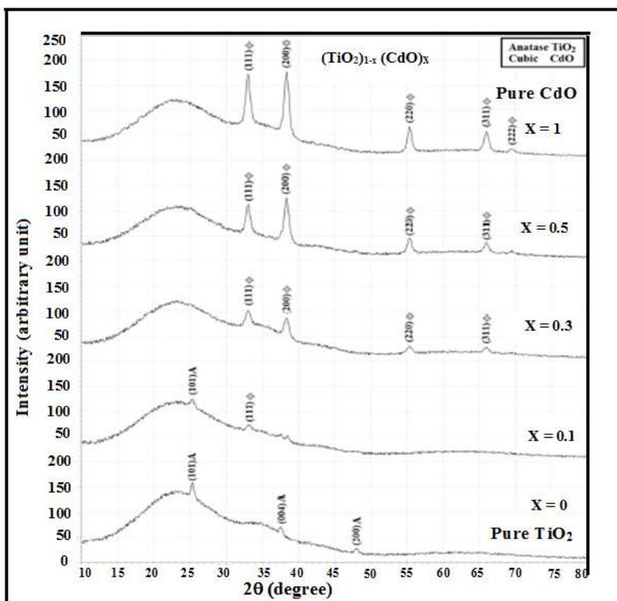
Fig.(2) X-Ray Diffraction for  $(\text{TiO}_2)_{1-x}(\text{CdO})_x$  Thin Films at 500 k
