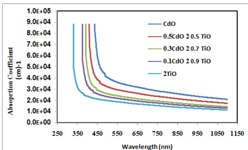
Fig.(4) :Variation of absorption coefficient as a function of wavelength for  $(\text{TiO}_2)_{1-x}(\text{CdO})_x$  films at  $T_a = 500 \text{ k}$
