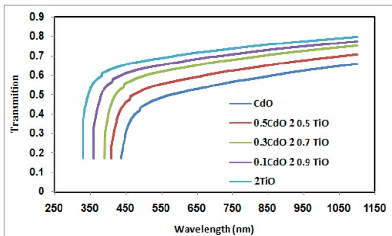
Fig.(3): The transmission spectra of  $(\text{TiO}_2)_{1-x}(\text{CdO})_x$  thin films annealed at  $T_a = 500 \text{ k}$
