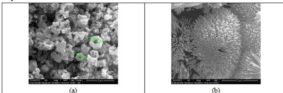
**Fig3:** SEM micrographs of ZnO nanopowder synthesized by Sol Gel(a) and Dry Mechano- chemical methods(b)
