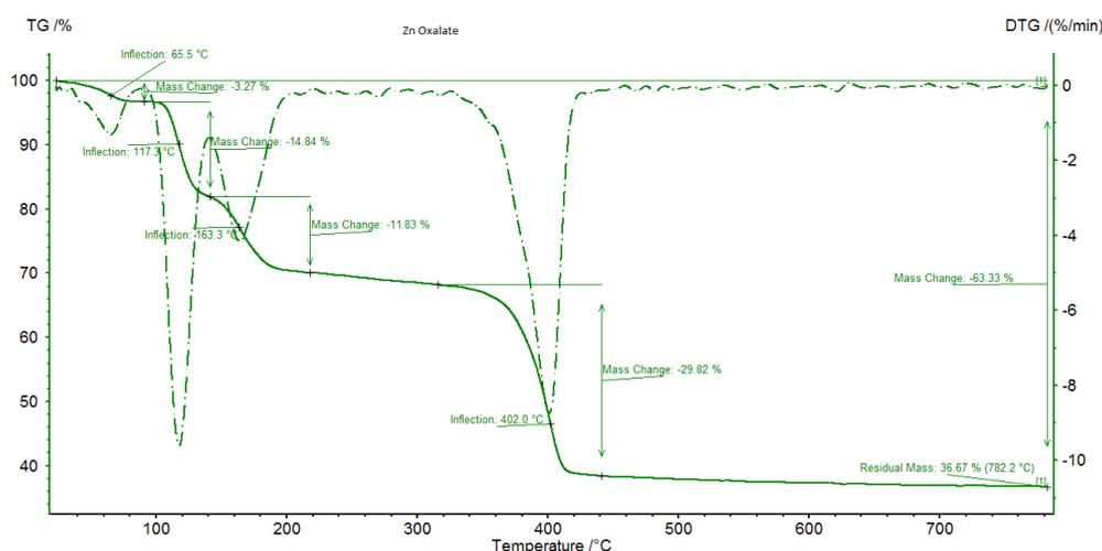
**Fig2.2:** TG and DTG curves of Zinc oxalate with weight loss% at various temperatures.
