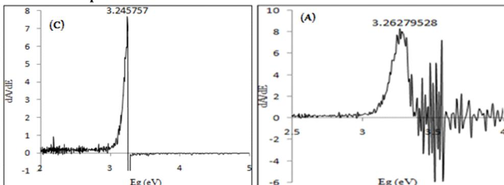
**Fig 4.** First derivative of UV-Vis Absorption Spectra for the ZnO samples by Sol Gel(A) and Dry Mechano-chemical methods(B)
