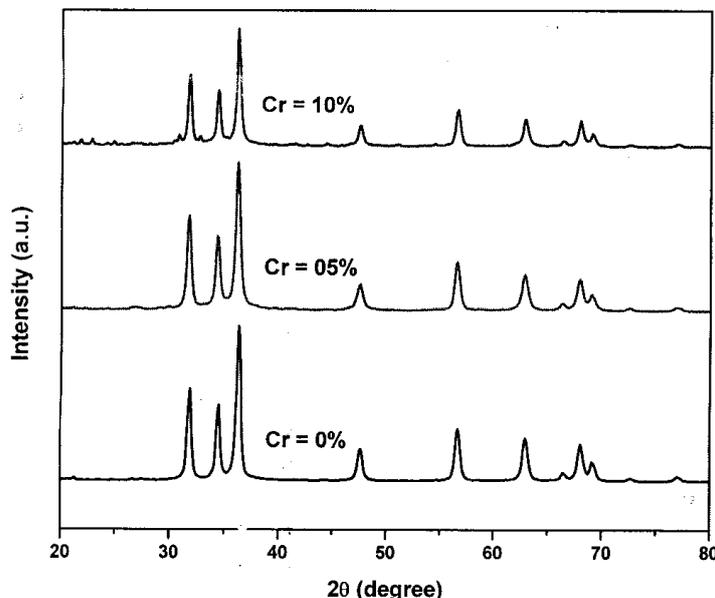
**Figure 1.** XRD pattern of Pure ZnO and Cr-doped ZnO nanoparticles of varying Cr dopant concentration.
