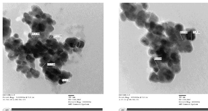
Figure 2(a). TEM image of ZnO sample. Figure 2(a). TEM image of 5% Cr doped ZnO sample.
