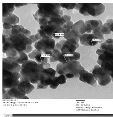
Figure 2(c). TEM image of 10% Cr doped ZnO sample.
