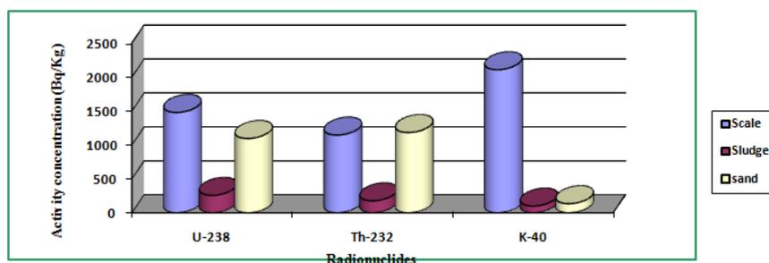
**Figure 4:** Comparison of average activity concentration of radionuclides found in Scale, sludge and sand
