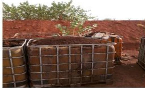
**Sand extracted from vessel and put in drums in special closed area**
