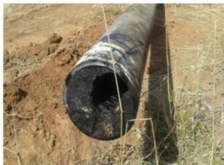
**An abandoned pipeline due to heavy scale formation**
