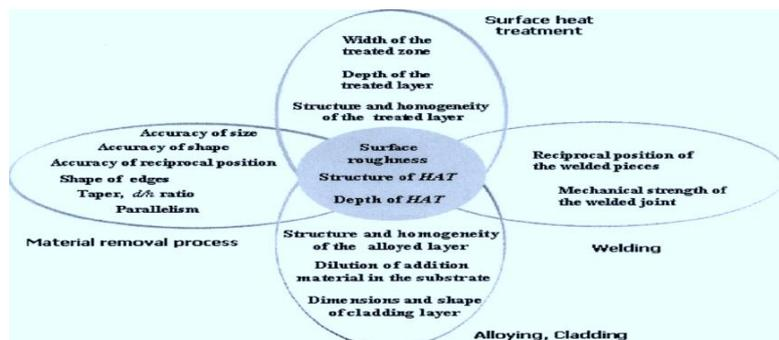
Figure 0: Objective functions of the laser assisted material processing
