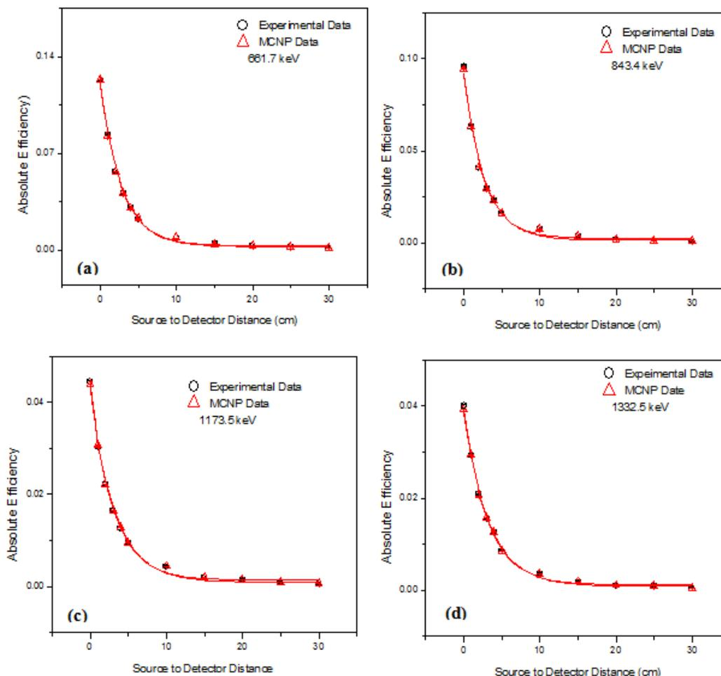
**Figure 2.** Absolute efficiency at different source to doctor distance in comparison with MCNP value
