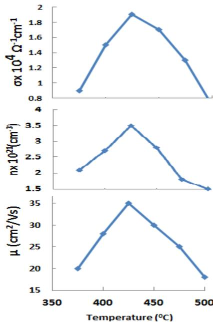
Fig.3 Variation of conductivity, carrier concentration and Hall mobility of doped film ( $S_nO_2:F$ ) at deposited at different substrate temperature.
