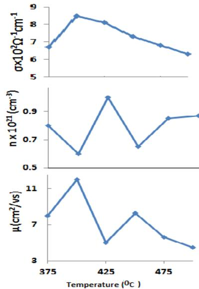
Fig. 2. Variation of conductivity, carrier concentration and Hall mobility of undoped film ( $S_nO_2$ ) at deposited at different substrate temperature.
