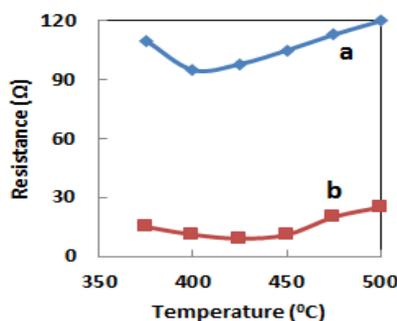
**Fig. 1.** Variation of sheet resistance with as deposited at different temperature of (a) undoped and (b) fluorine doped  $SnO_2$  thin films.
