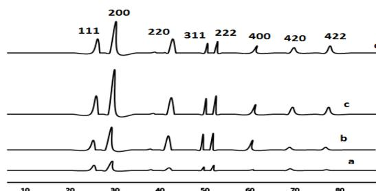
**Fig. 1.** X-ray pattern of as deposited  $CuInTe_2$  thin film prepared at temperature a) 300°C, b) 325°C, c) 350°C and 375°C
