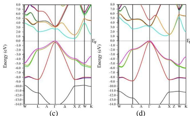
**Fig.3.** Band structures using GGA with SOI for (a) BN (b) BP (c) BAs (d) BSb
