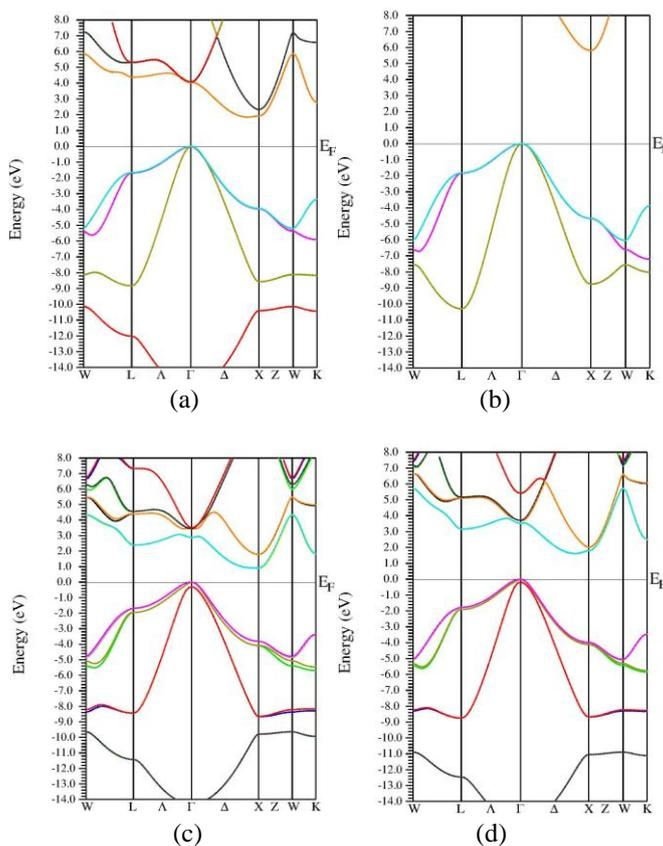
**Fig.4.** Band structures using mBJ with SOI for (a) BN (b) BP (c) BAs (d) BSb
