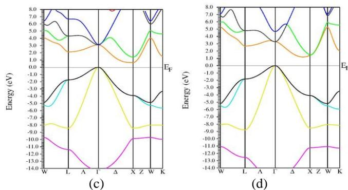
**Fig.1.** Band structures using GGA without SOI for (a) BN (b) BP (c) BAs (d) BSb
