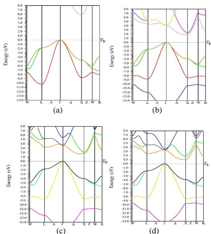
**Fig.2.** Band structures using mBJ without SOI for (a) BN (b) BP (c) BAs (d) BSb
