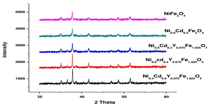
**Figure1:** Structural properties of Ni<sub>1-x</sub> Cd<sub>x</sub> Y<sub>y</sub> Fe<sub>2-y</sub> O<sub>4</sub> by XRD
