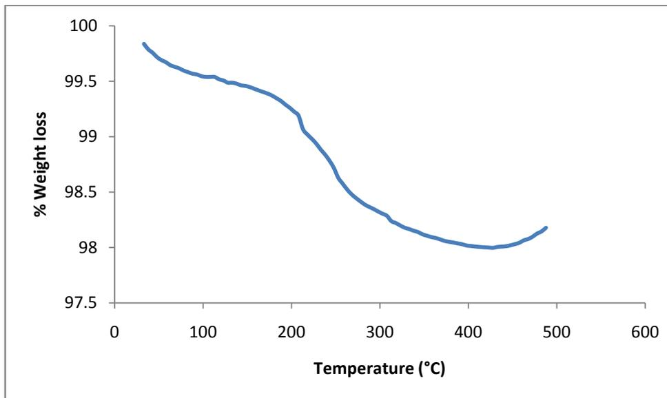
**Figure 5:** TGA curve for  $Ni_{0.8}Cd_{0.2}Y_{0.075}Fe_{1.925}O_4$  nanoferrites
