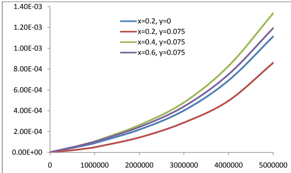
**Figure4:** Variations of AC Conductivity with frequency of  $Ni_{1-x}Cd_xY_yFe_{2-y}O_4$  nanoferrites
