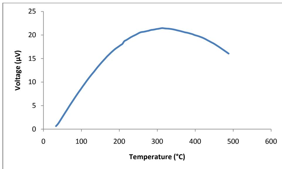
**Figure 6: DTA curve for  $Ni_{0.8}Cd_{0.2}Y_{0.075}Fe_{1.925}O_4$  nanoferrites**
