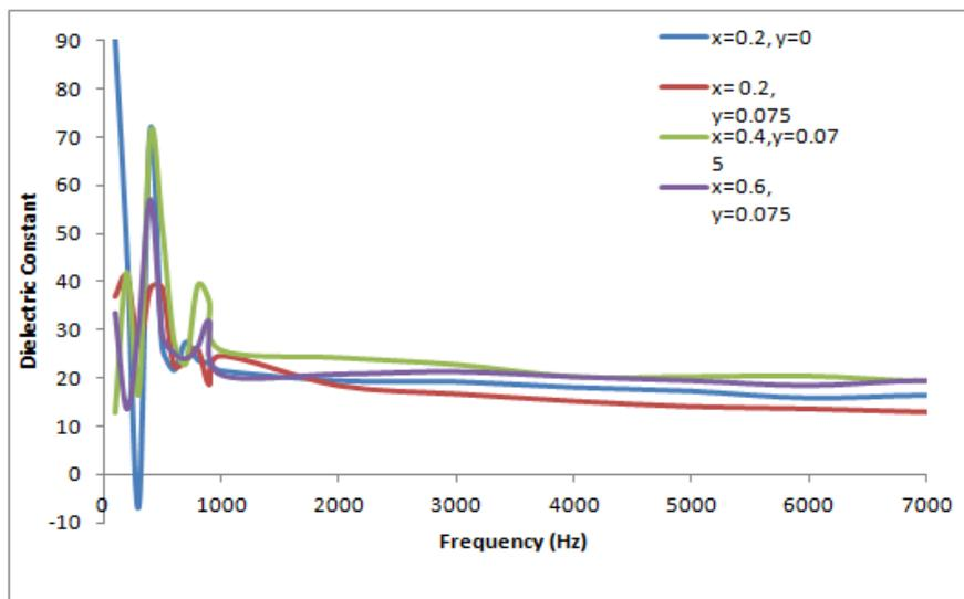
**Figure 2:** Variations of dielectric constant with frequency of  $Ni_{1-x}Cd_xY_yFe_{2-y}O_4$  nanoferrites
