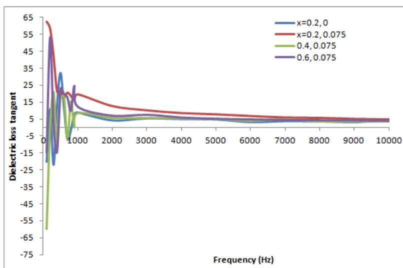
**Figure3:** Variations of dielectric loss with frequency of  $Ni_{1-x}Cd_xY_yFe_{2-y}O_4$  nanoferrites
