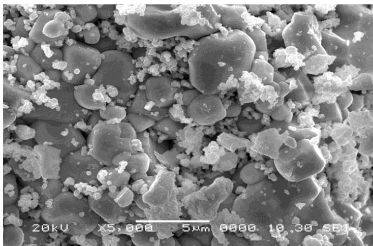
**Fig. 3:** Scanning Electron Microscopy of pure Lead Titanate sample
