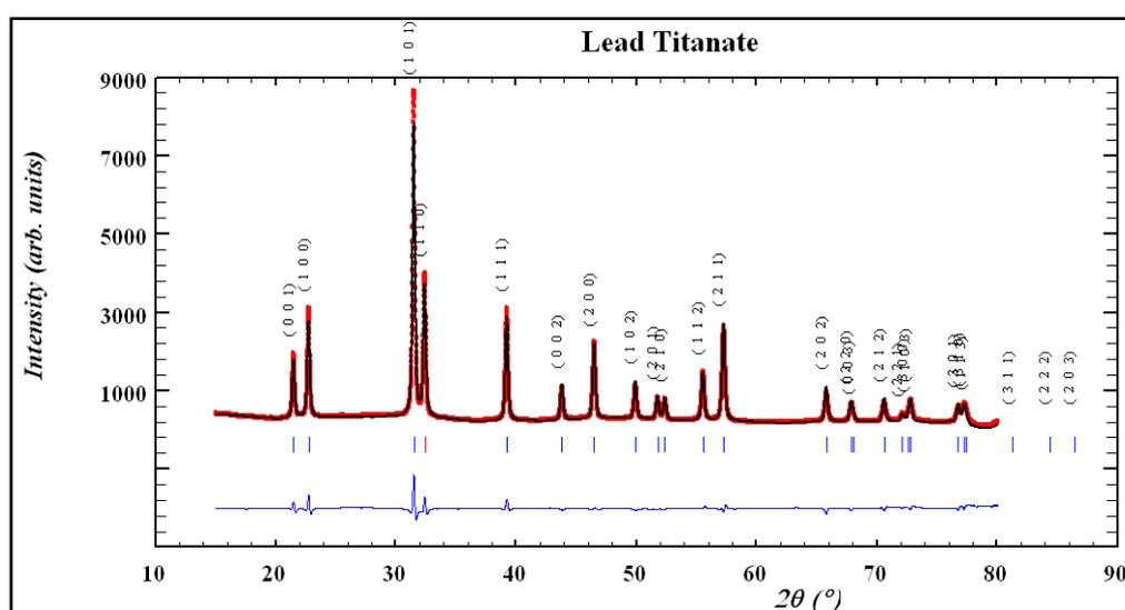
Fig. 2: Rietveld refined XRD pattern for the  $PbTiO_3$  sample. The circles represent experimental points and the solid line represents Rietveld refined data. The bottom line shows the difference between the experimental and refined data. The marked  $2\theta$  positions are the allowed Bragg peaks.
