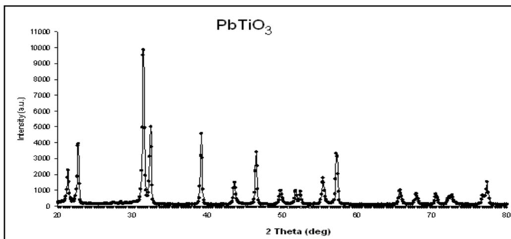
Fig. 1. The XRD pattern of  $PbTiO_3$  sample.
