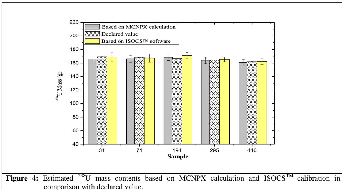
**Figure 4:** Estimated <sup>238</sup>U mass contents based on MCNPX calculation and ISOCS™ calibration in comparison with declared value.
