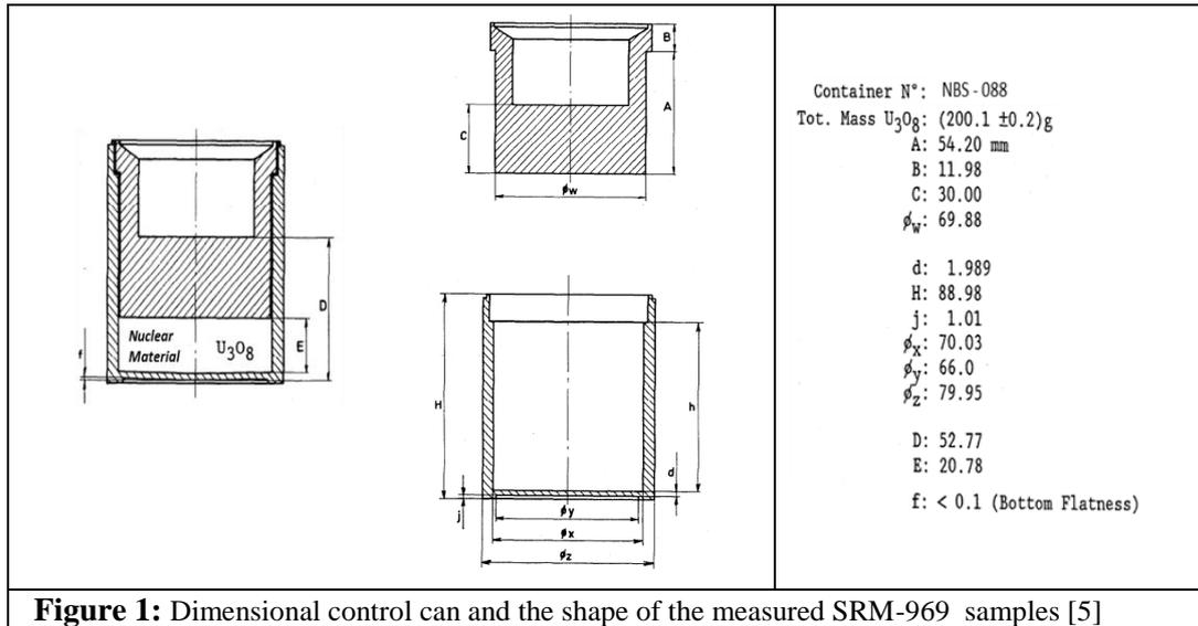
**Figure 1:** Dimensional control can and the shape of the measured SRM-969 samples [5]
