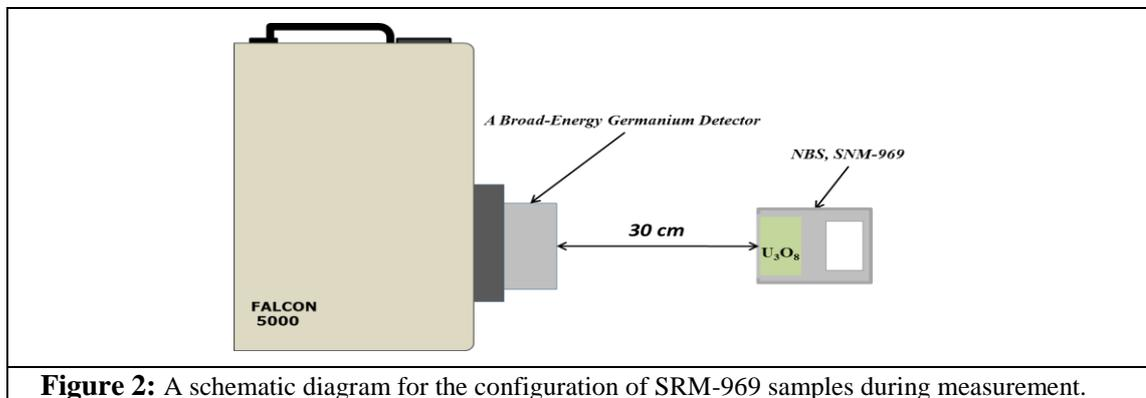
**Figure 2:** A schematic diagram for the configuration of SRM-969 samples during measurement.
