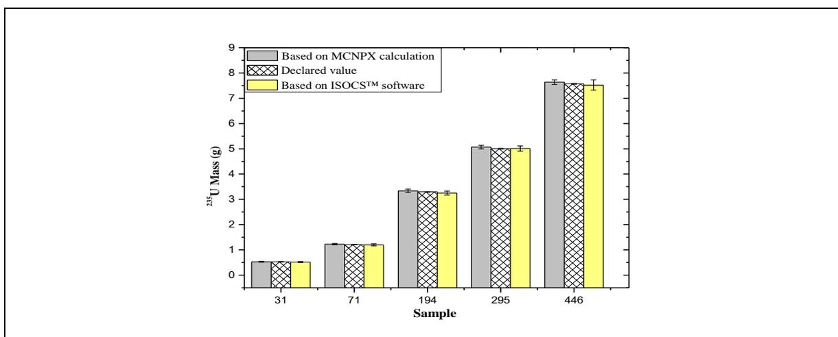
**Figure 3:** Estimated <sup>235</sup>U mass contents based on MCNPX calculation and ISOCS™ calibration in comparison with declared value.
