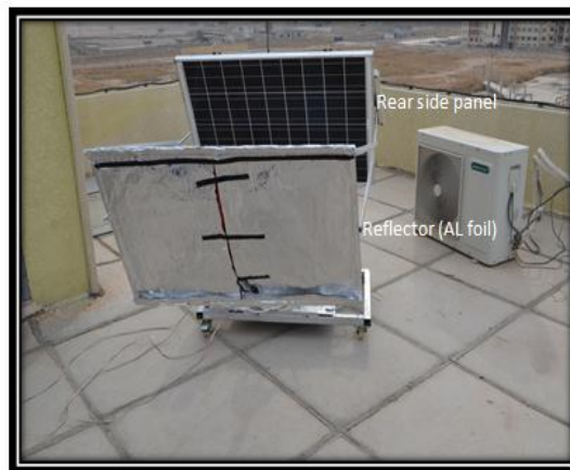
Fig. 14: One axis tracker including (in front, rear side panel and reflector) arrangement.
