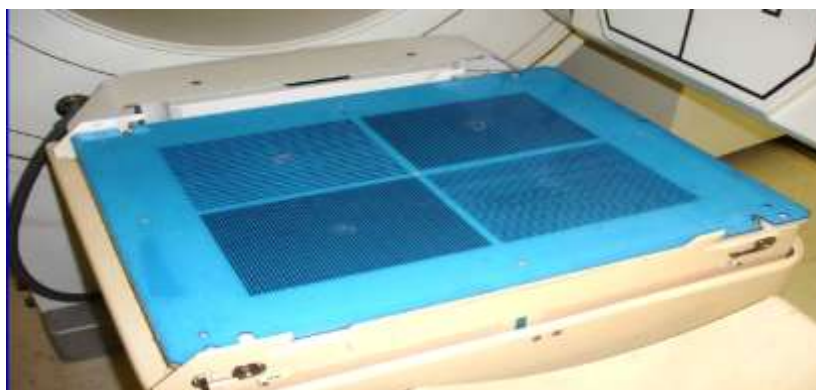
Fig 1. gamma camera with a quadratic bar phantom placed on top of the gamma camera detector
