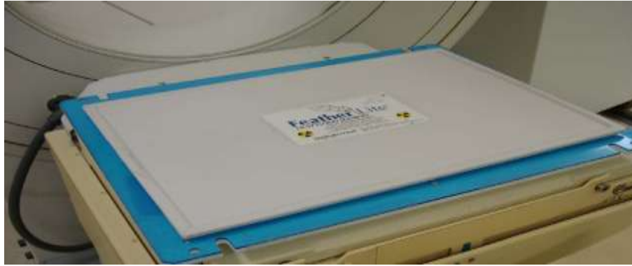
Fig2. gamma camera with a quadratic bar phantom placed on top of the gamma camera detector and radioactive source on top of the quadratic phantom for transmission images
