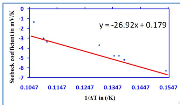
**Figure 1:** Plot of Seebeck coefficient versus Reciprocal of Temperature
