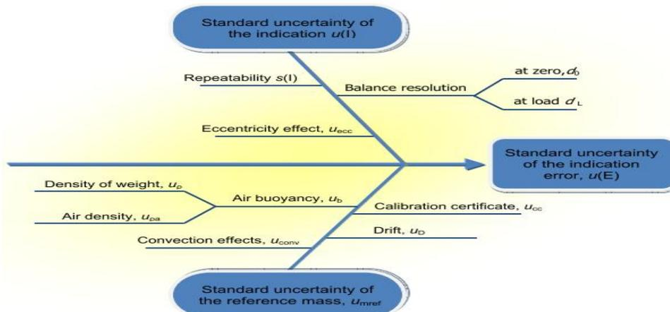
**Figure1** Ishikawa diagram of uncertainty components in the calibration of the balance
