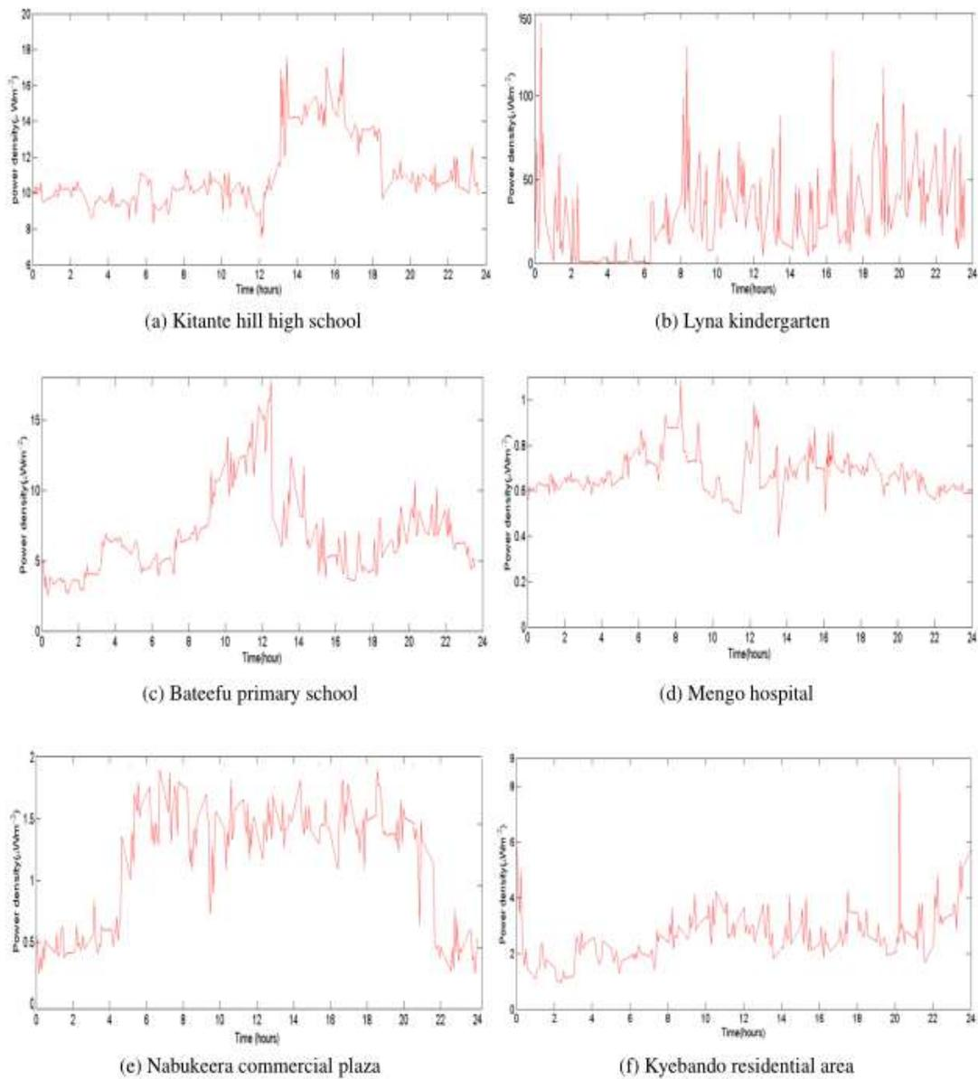
**Figure 3:** GSM1800 temporal exposure
