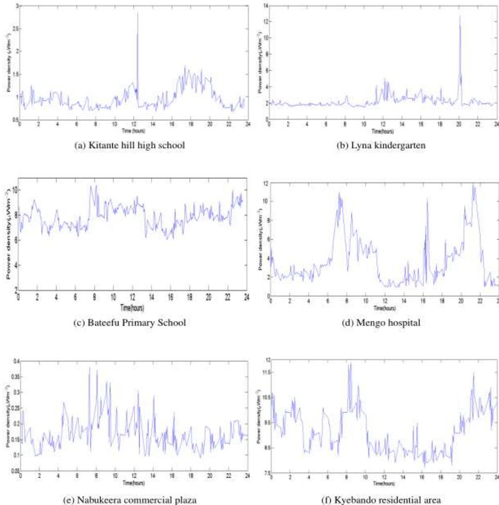
**Figure 2:** GSM900 temporal exposure
