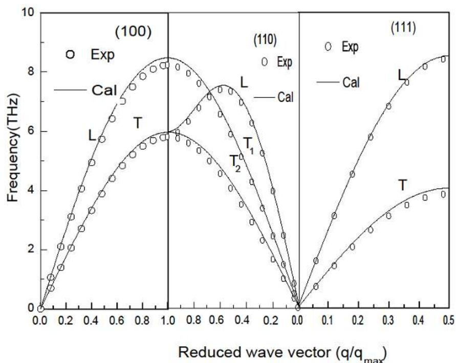
**Fig1.** : Phonon dispersion curves of Ni<sub>0.76</sub>Fe<sub>0.24</sub> alloy
