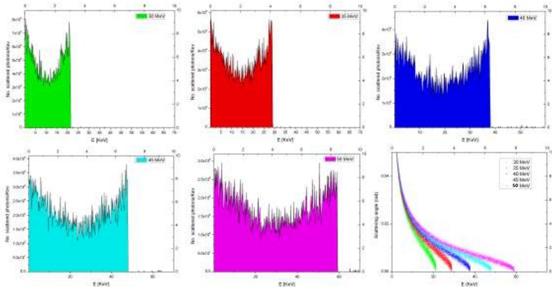
**Figure (3).** Emitted X-ray photons from electron pulse collision with Ti:Sapphire laser pulse. The first 5 sub figures represent the angular distributions at different energies. The last sub figure represents the energy spectrum at such electron energies
