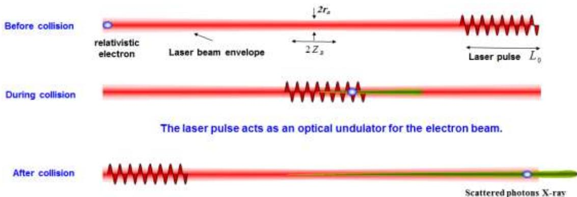
**Figure (1).** Generation of monochromatic X-ray radiation form Inverse Compton Scattering.
