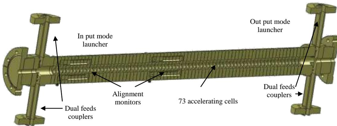
**Figure (2):** Cut view of X-band structure showing the mode launchers and wakefield monitors.
