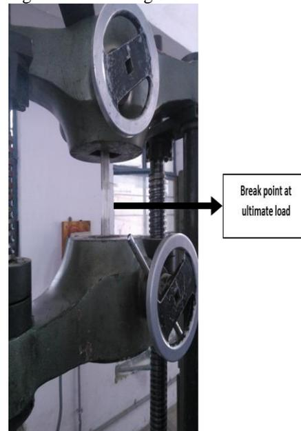
Fig.3.2 Laminate during Tensile Test
