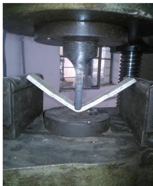
Fig.3.4 Laminate after Bending Test
