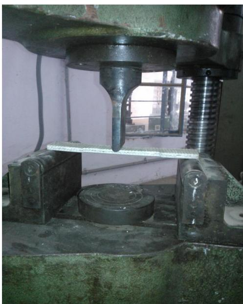
Fig.3.3 Laminate before Bending Test
