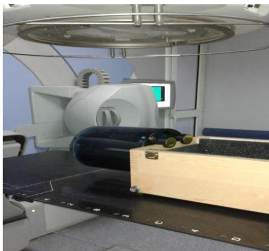
Figure (2): Catphan phantom for image quality tests
