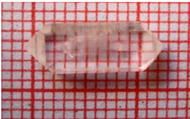
Fig.1. Photograph of as grown crystal of ZLMHCl
