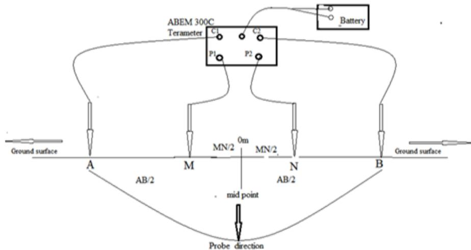
**Figure 2.1:** Schematic Diagram of schlumberger array field method
