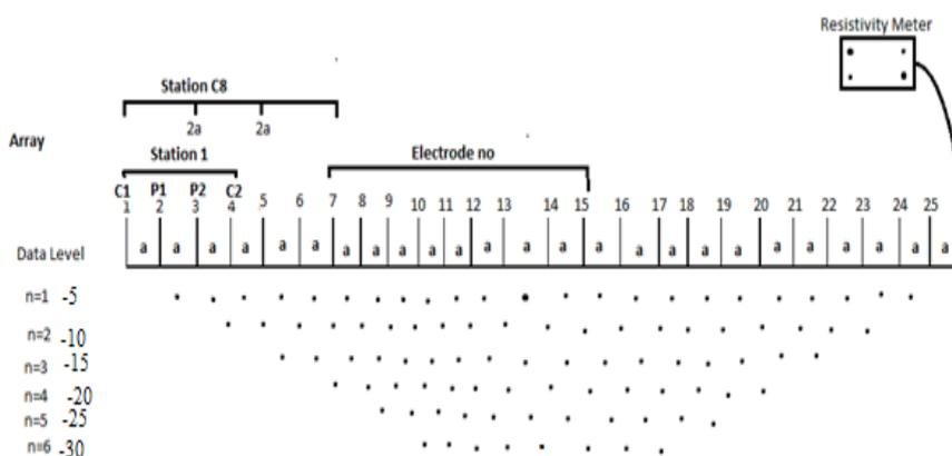
Figure 2.3: The arrangement of electrodes for 2-D Imaging. (The dots indicate midpoint-point).
