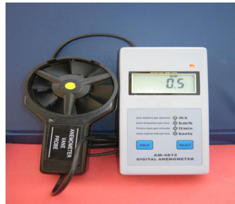
Fig 1.4 Digital Anemometer for Wind Speed Measurement
