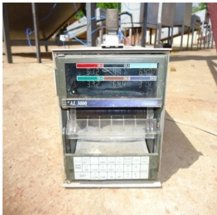
Fig 1.3 Digital thermocouple data logger
