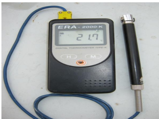
Fig 1.5: Digital Thermometer for Ambient Temperature Measurement
