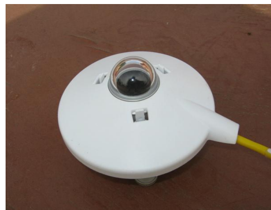
Fig 1.6: Pyranometer for Global Solar Radiation Measurement
