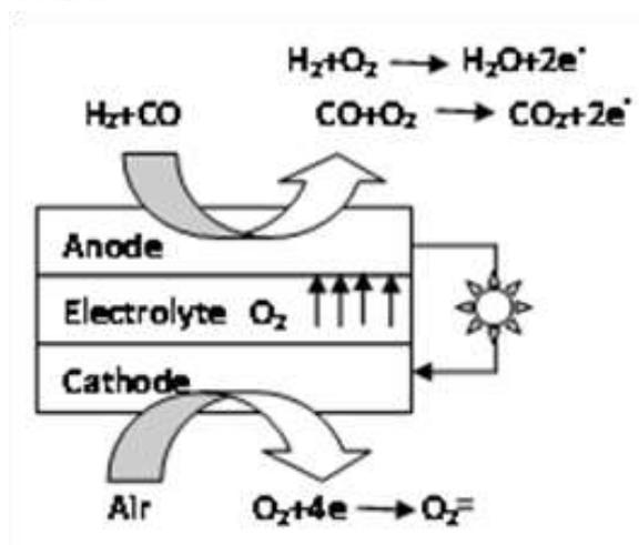
Fig. 1 Solid Oxide Fuel Cell
