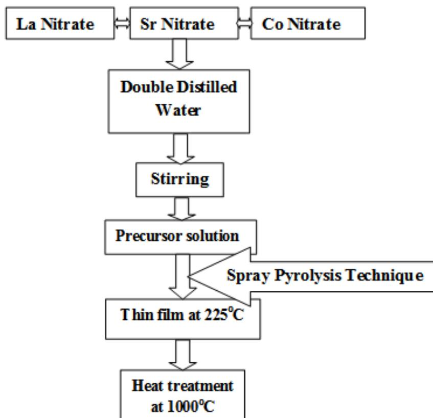
**Fig. 2** Flow chart of spray deposition technique
