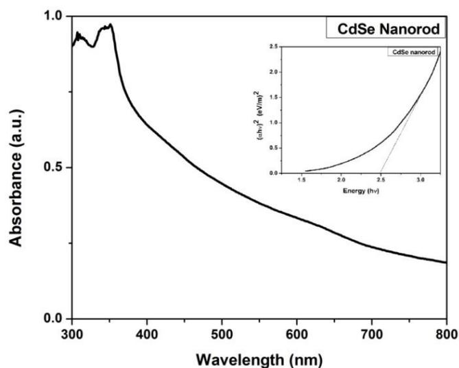
Fig. 3 Optical absorption spectra (band gap determination at the inset) of the CdSe nanorods.
