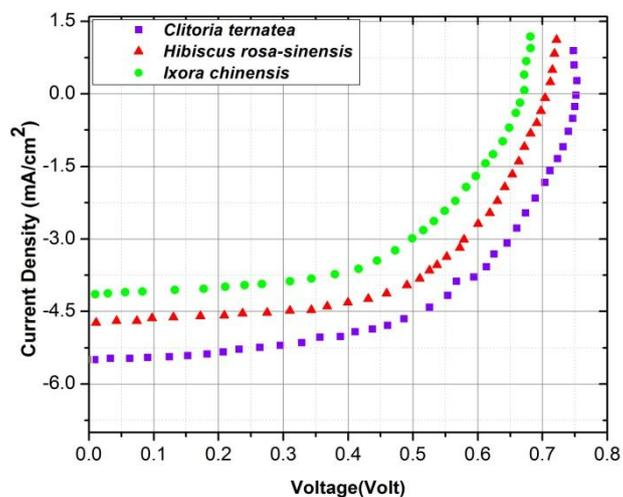
Fig. 5a. Current density (J) - Voltage (V) characteristics of DSSCs.
