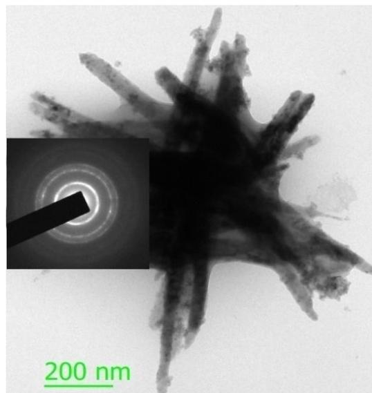
Fig. 2 TEM and SAED image of CdSe nanorod.
