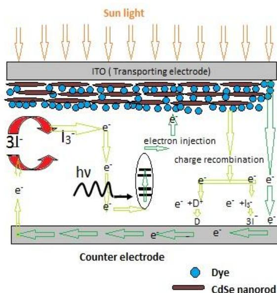
Fig. 1 The schematic diagram of fabricated DSSC.
