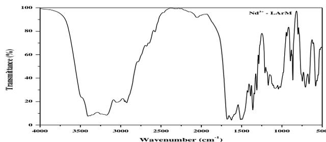
Fig 4. FTIR spectrum of Pure and LArM single crystals
