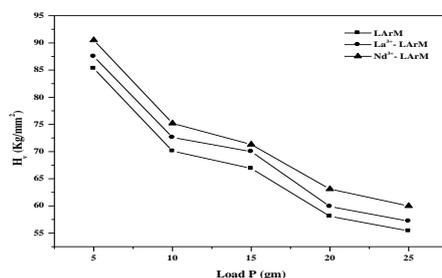
Fig 5. Variation of hardness with applied load
