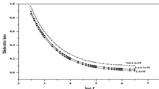
Fig 7. Variation of dielectric loss of pure and doped LArM
