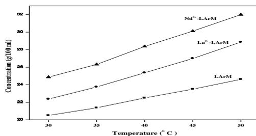
Fig. 1 Solubility curves of pure and doped LArM crystals
