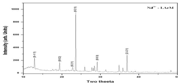
Fig 3. XRD pattern of Pure and Doped LArM single crystals
